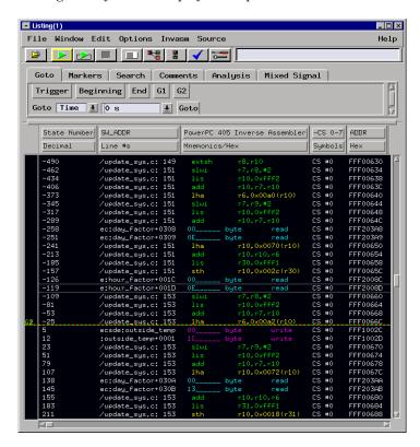
The inverse assembler is loaded when state configuration files are loaded, but it can also be loaded into a Listing display using the Invasm menu. The name of the inverse assembler file is I405E.
