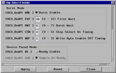
For the PPC405 inverse assembler to properly handle burst cycles additional information must be provided by the user. The ~PerBlast signal on the PPC405 Peripherals Bus indicates that a burst cycle is in progress, but there is no signal indicating the point in the cycle where the address and data are valid. The number of wait states, the Chip-Select-On-Timing, and the Write-Byte-Enable-Off-Timing are needed to determine this address/data valid
