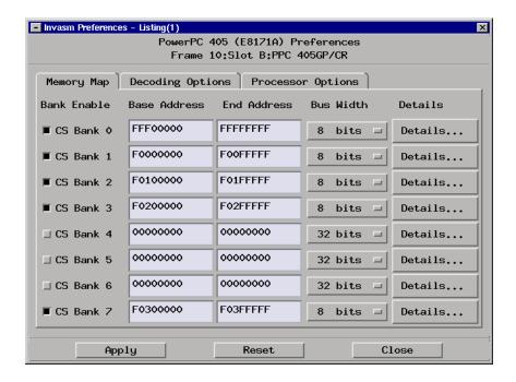
**Bank Enable.** Enable the banks for all of the chip selects, and only those chip selects, being used in the system; otherwise, the inverse assembler may not function correctly. These enables are required because with the PPC405 most chip selects can be configured to be general purpose I/O (GPIO) signals.
